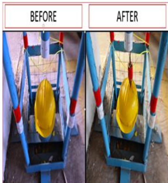
Pict.2: Safety Helmet Testing (Before & After)
