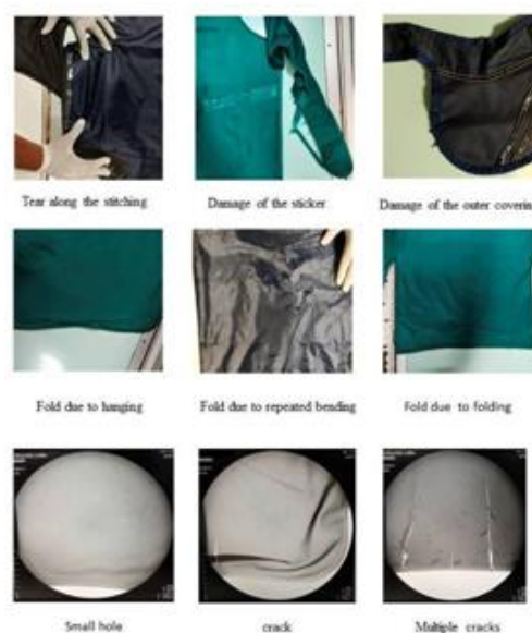
Figure 4: The picture gallery of the visual, tactile, and fluoroscopic defects on the radioprotective apparel
