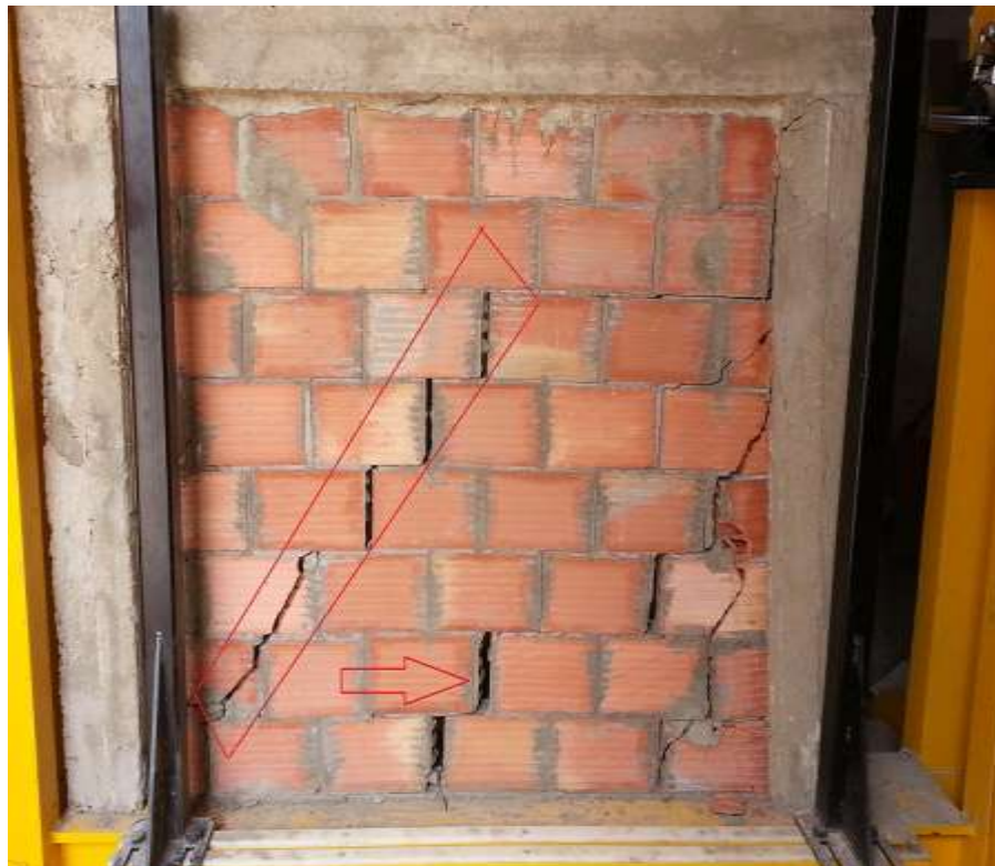
Figure 3: Cracking at the joints
