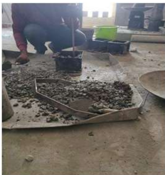
Figure 6: Preparation of fresh concrete
