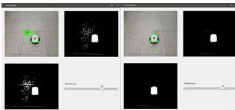
Figure 9: Feature extraction, locating the centroid of the desired object
