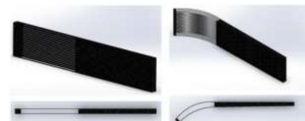
Figure 5: Endplate CAD with SMA wires
