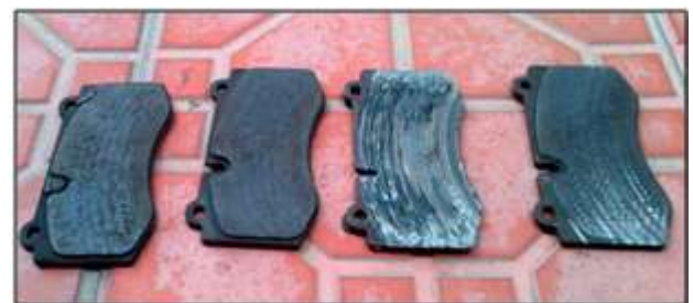
Figure 2: Behaviour of Brake pads under Wear
