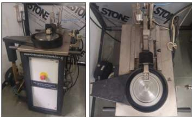
Figure 4: Work piece setting on Pin on Disc
