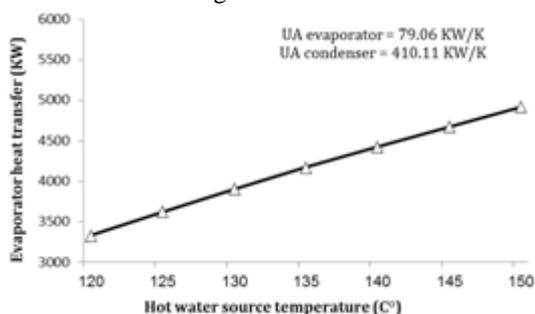
Figure 13: Effect of hot water source temperature variation on evaporator heat transfer
