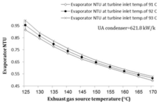
Figure 7: Variations of evaporator NTU versus source temperature
