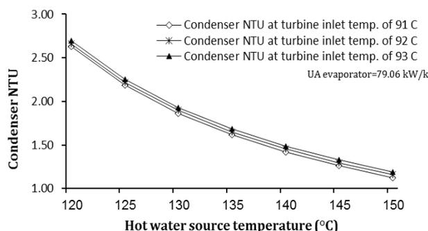
Figure 17: Variation of condenser NTU versus source temperature
