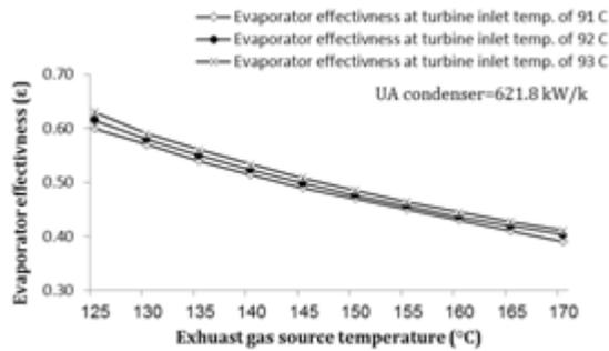
Figure 6: Variations of evaporator effectiveness versus source temperature
