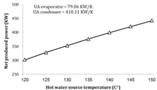
Figure 10: Effect of hot water source temperature variation on net output power.
