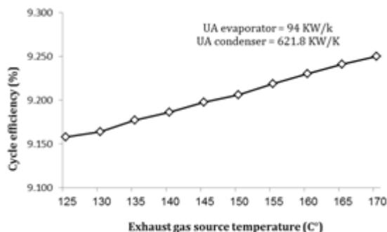
**Figure 3:** Effect of exhaust gas source temperature variation on cycle efficiency
