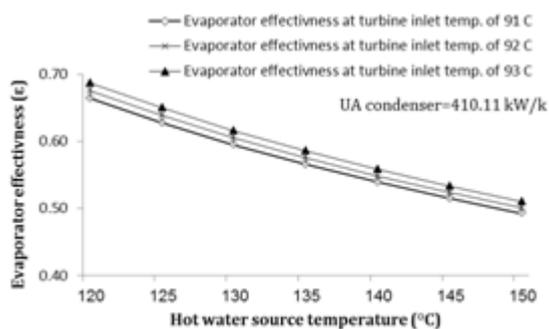
Figure 14: Variations of evaporator effectiveness versus source temperature
