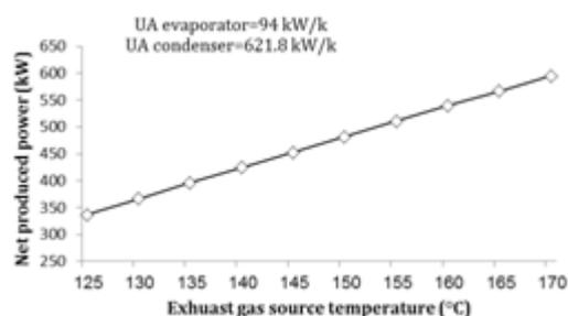
**Figure 2:** Effect of exhaust gas source temperature variation on net output power
