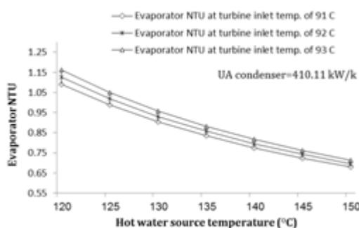
Figure 15: Variations of evaporator NTU versus source temperature.
