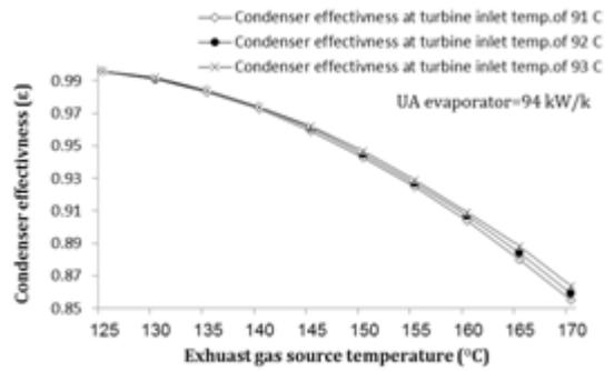
Figure 8: Variation of condenser effectiveness versus source temperature
