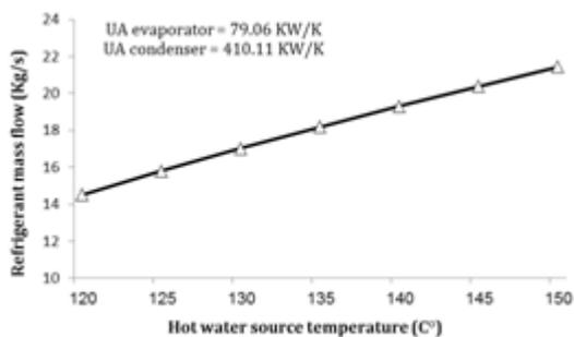
Figure 12: Effect of hot water source temperature variation on refrigerant mass flow
