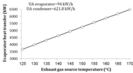
Figure 5: Effect of exhaust gas source temperature variations on evaporator heat transfer
