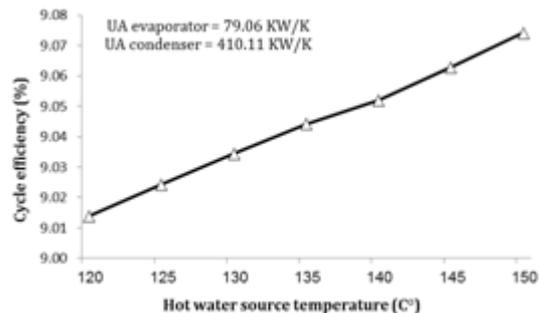
Figure 11: Effect of hot water source temperature variation on cycle efficiency
