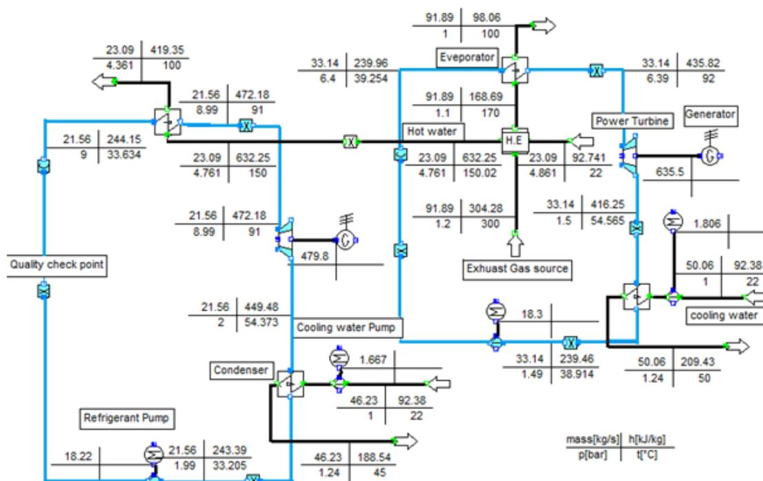
**Figure 1:** Direct electricity generation by R - 123, R245fa Cascade Organic Rankine cycle model
