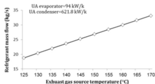
**Figure 4:** Effect of exhaust gas source temperature variation on refrigerant mass flow
