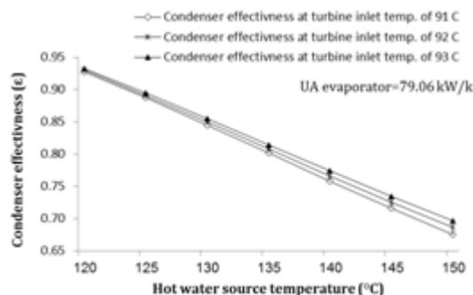
Figure 16: Variation of condenser effectiveness versus source temperature
