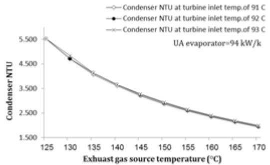
Figure 9: Variation of condenser NTU versus source temperature
