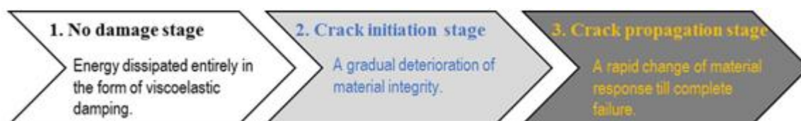
Figure 3: Evolution of damage linked to the fatigue of binders
