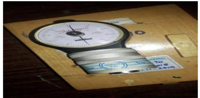
Figure 24: Durometer
