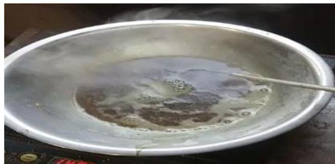
Figure 17: Heating the Natural resin (Gum Rosin)
