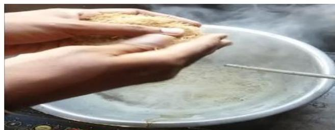
Figure 18: Adding Coconut fiber into the natural resin
