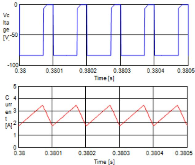
Figure 11: Simulation results of the input current and voltage across the diode  $D_1$ .
