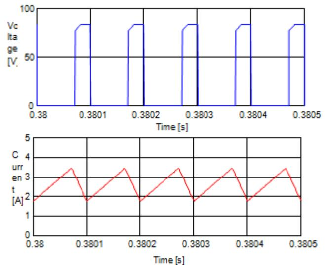
Figure 10: Simulation results of the input current and voltage across the power switch S.
