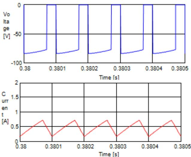
Figure 12: Simulation results of the output current inductor ( $i_{L2}$ ) and voltage across the diode  $D_2$
