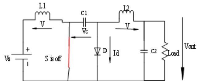
Figure 4: Mode 2 operation of CUK converter
