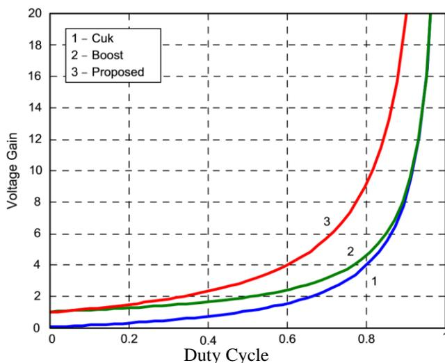
**Figure 6:** Static voltage conversion ratio as a function of duty-cycle.
