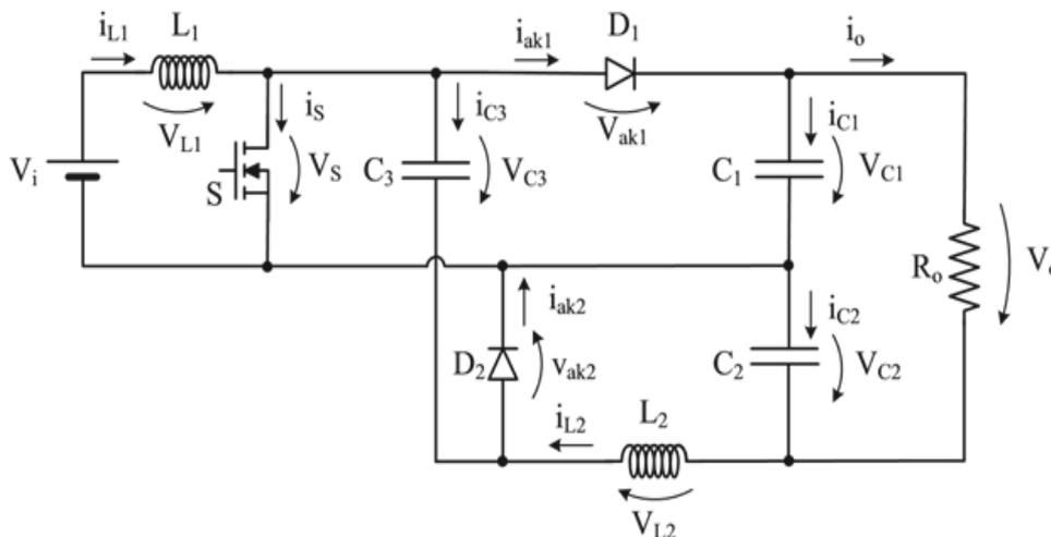
**Figure 5:** Proposed hybrid DC-DC converter with extended voltage ratio
