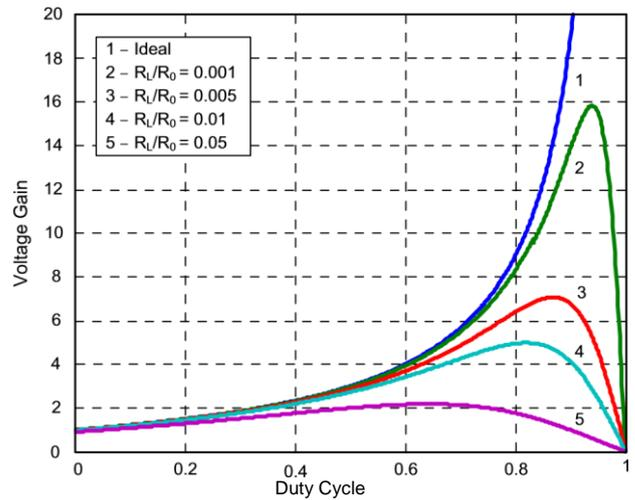
Figure 8: Static voltage conversion ratio as a function of duty cycle considering inductor losses
