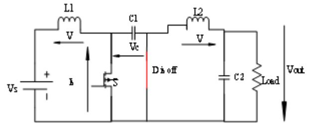
Figure 3: Mode 1 operation of CUK converter
