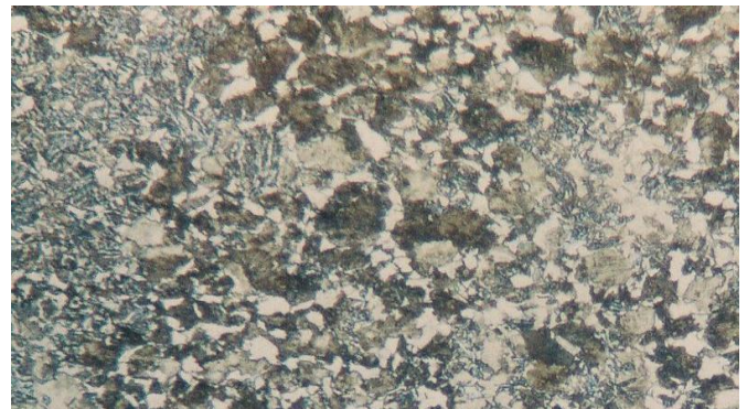
Figure 3: Microstructure of Normalized AISI 4140 alloy steel (500X)
