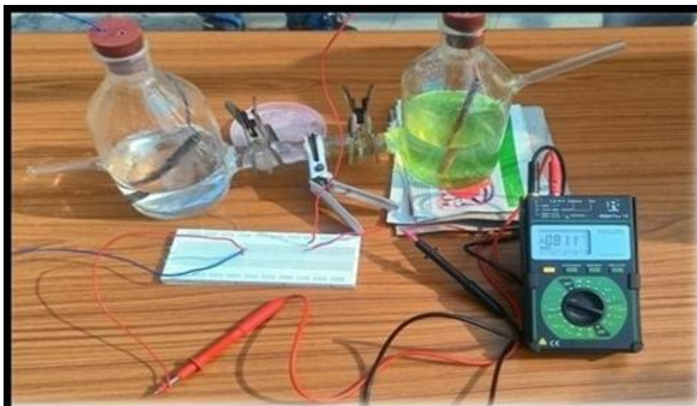
Figure 4: Working of Prototype of Bio-photovoltaic Cell
