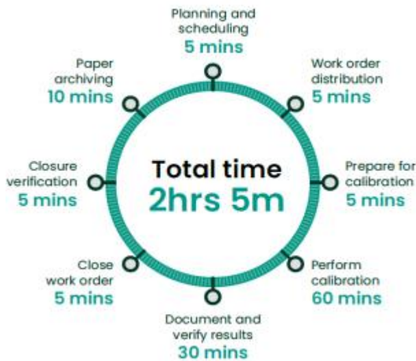
Figure 1: Traditional calibration process.
