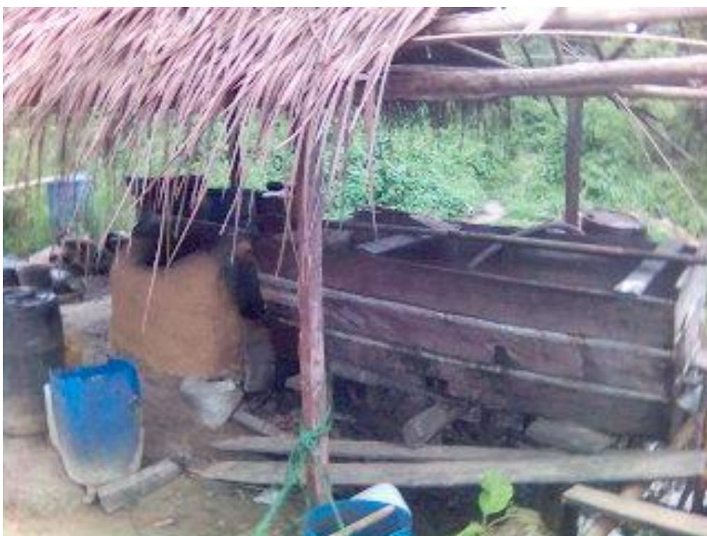
Figure 3: Cooling chamber made of locally fabricated large bowl of water through which the lead pipe passes to a dripping point.
