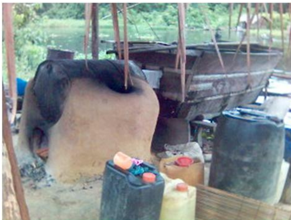
Figure 5: A typical brewing unit along the coastal areas of Bayelsa State with rubber containments
