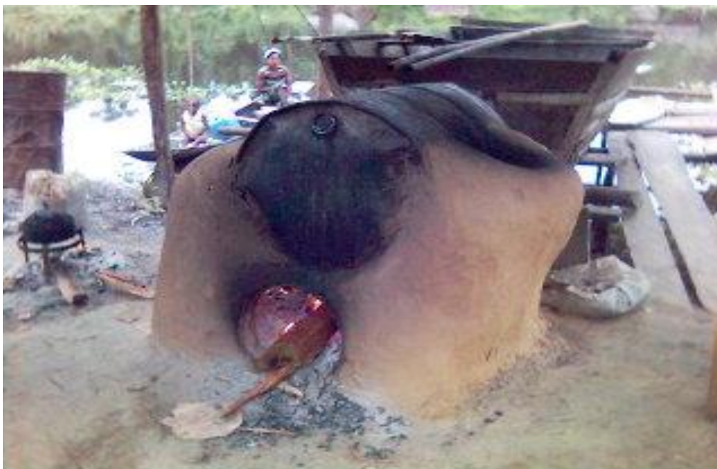
Figure 2: Heating chamber made of horizontally positioned drum place over a heating source
