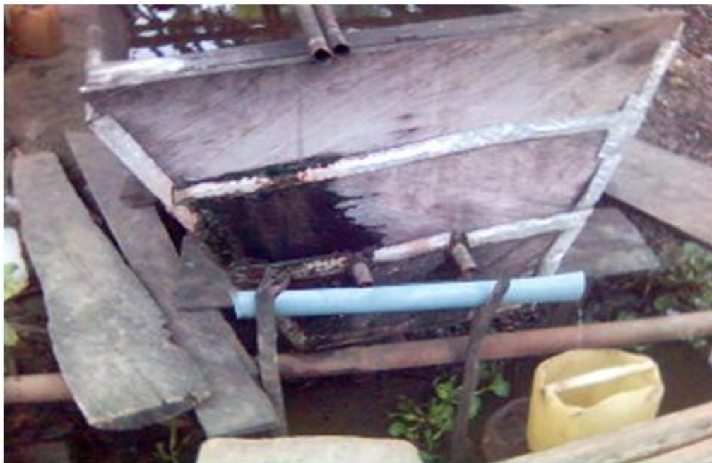
Figure 4: Dripping or collection point showing the condensed alcohol vapour
