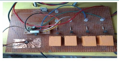
Another control system is used for the sprinkler system i.e. to provide interrupted water supply to the floor, so for this purpose only one relay set is used which provide the flow of water in the discontinuous manner.
