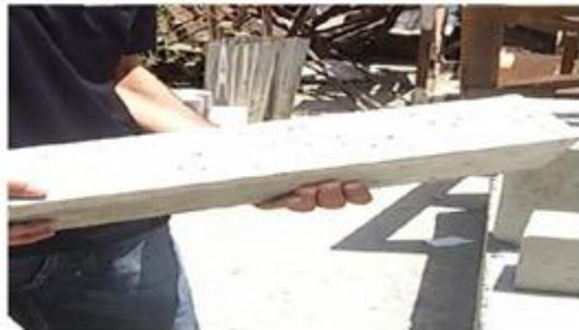
Beam Specimen for Flexure Test
