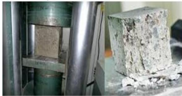
Compressive test of sample
