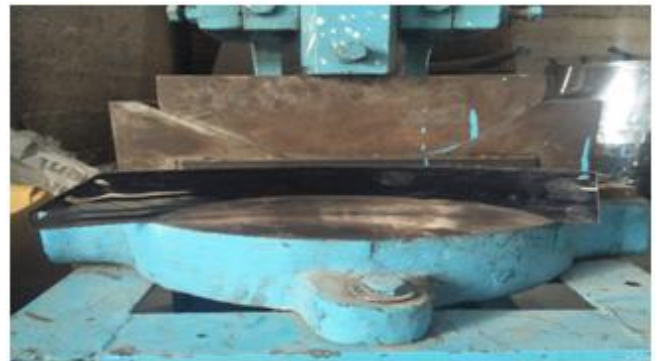
Figure 4.4: Blade after Die Pressing
