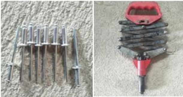
Figure 4.7: Rivet (left) and Rivet Gun (right)
