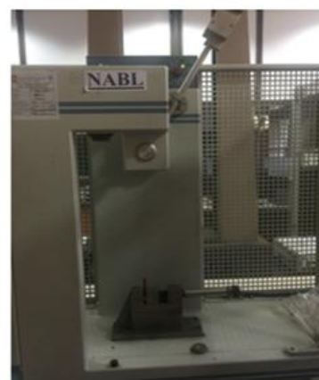
Figure 4: Impact strength testing of specimens using Izod type impact testing machine
