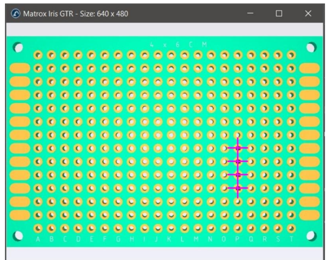
Figure 9: Target detection on PCB surface
