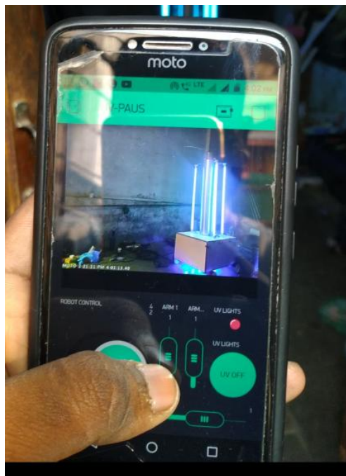
Figure 6.2: The Blynk Mobile Application wireless remote-control interface of UV-PAUS Robot with LIVE streaming
