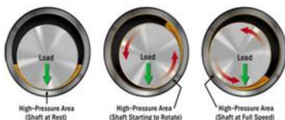
Figure 2: Hydrodynamic bearings
