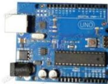
Figure 4: ARDUINO UNO Board
