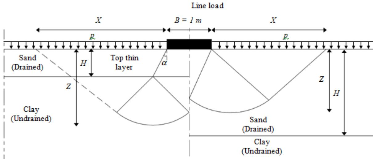
Figure 1: Problem notations and potential failure mechanisms
