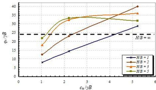
**Figure 3:** Bearing capacity of strip footing of sand overlying clay for various clay shear strength
