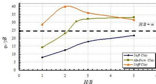
Figure 2: Bearing capacity of strip footing of loose sand overlying clay
