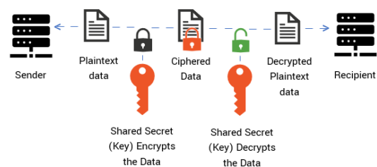
Figure 1: Symmetric encryption scheme
