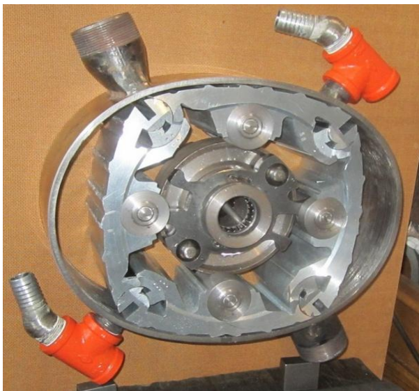
Photo C: Sample of a Quasiturbine stator executed from the computation results
