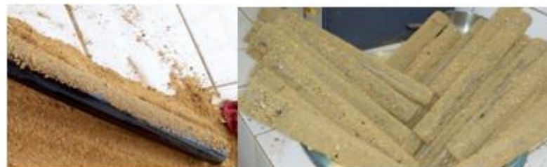
Figure 3: Raffia stems protected with the fluidify bitumen
