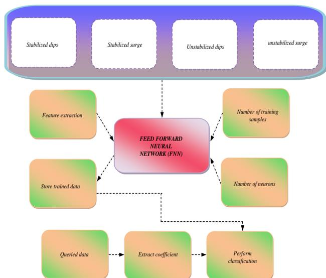
**Figure 4:** Schematic diagram of the PQ prediction using FNN
