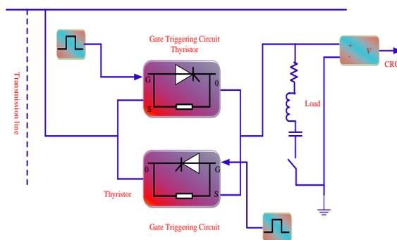
Figure 2: Usage of AC Voltage Controller Circuit
