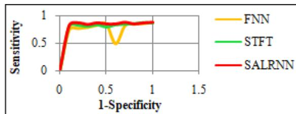
**Figure 10:** ROC of the PQ Detection and Classification Techniques
