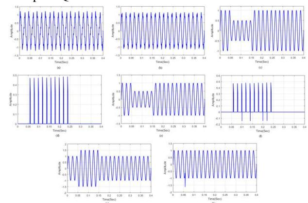
**Figure 7:** Detection results for single PQ event (a) Harmonics (b) Flicker (c) Interruption (d) Notch (e) Sag (f) Spike (g) Swell (h) Transient
