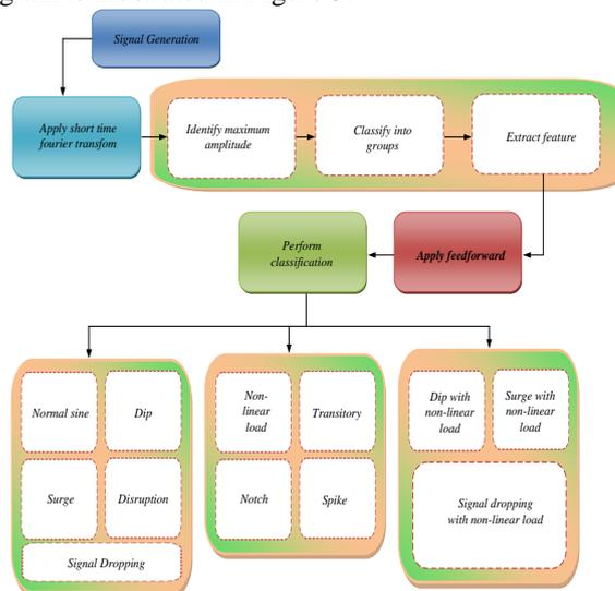
**Figure 5:** Schematic diagram of the PQ prediction using STFT
