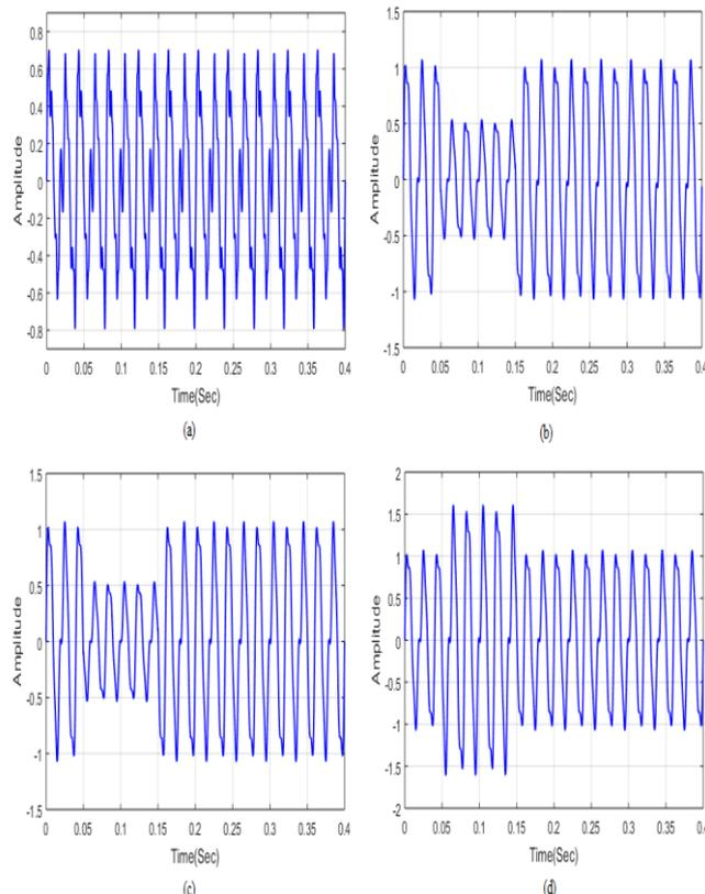
**Figure 8:** Detection results for multiple PQ events (a) Flicker with harmonics (b) Interruption with harmonics (c) Sag with harmonics (d) Swell with harmonics
