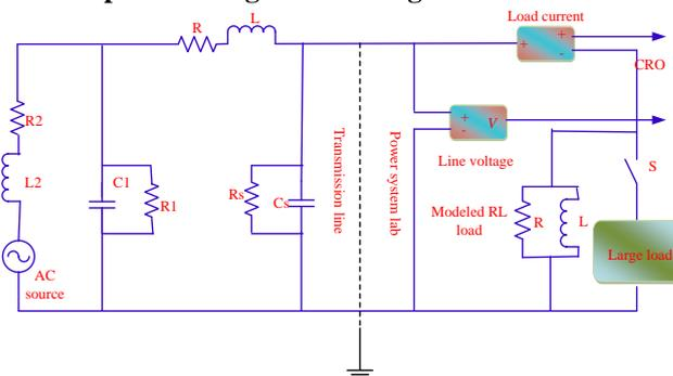
Figure 1: Abrupt Switching-on of a Large Load
