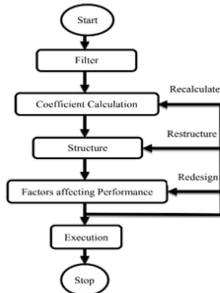
Figure 4: Design stages of digital FIR filters. [3]
