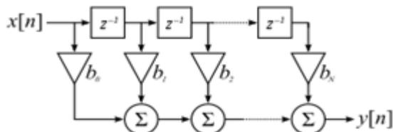
Figure 1: Finite impulse response (FIR) filter block diagram [8]
