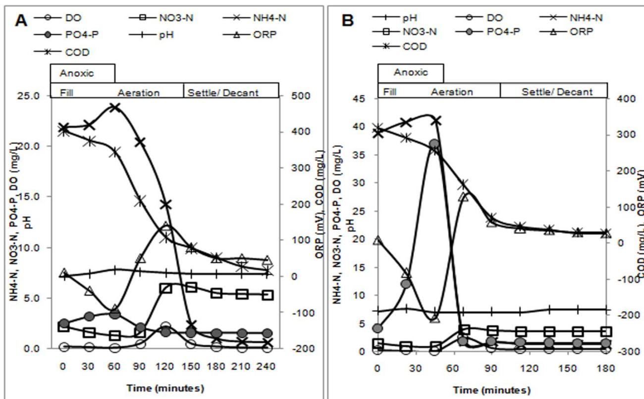
Figure 5: Time phase profiles of COD and nutrient removal with pH, DO, and ORP in SBR plants: (A) 3 MLD SBR plant (B) 120 MLD SBR plant
