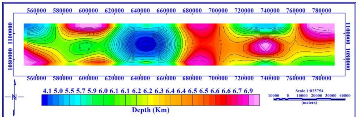
Figure 9: Aeromagnetic curie depth contour map of the study area (Km)
