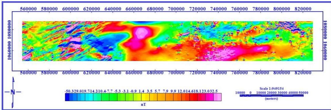
Figure 5: Residual of Upward continuation of aeromagnetic grid to 3000m altitude
