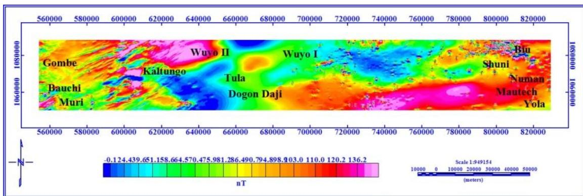
Figure 4: Reduced to Equator (RTE) of Aeromagnetic Map of the Study Area
