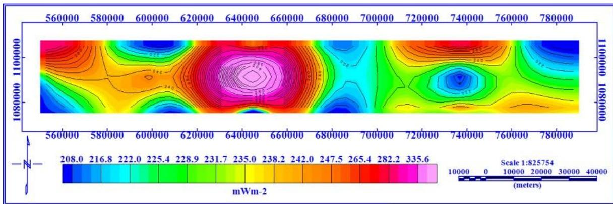
**Figure 11:** Aeromagnetic heat flow contour map of the study area ( $\text{mWm}^{-2}$ )
