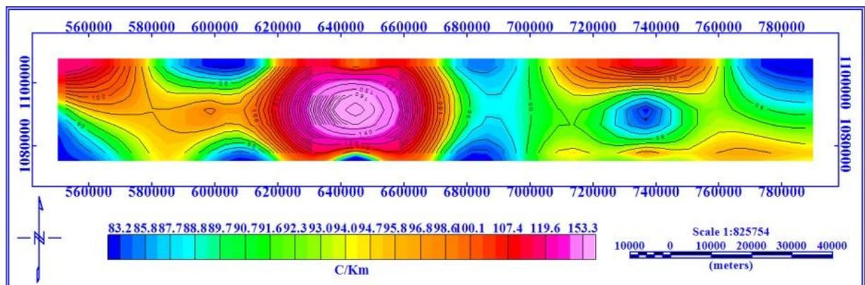
Figure 10: Aeromagnetic geothermal gradient contour map of the study area ( $^{\circ}\text{CKm}^{-1}$ )
