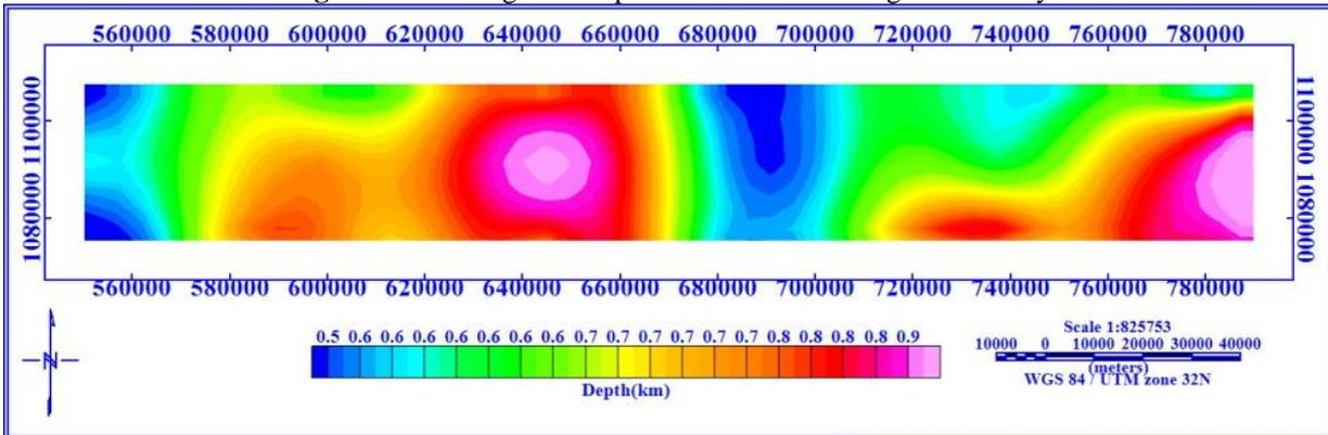
Figure 8: Aeromagnetic Depth to the top magnetic source map
