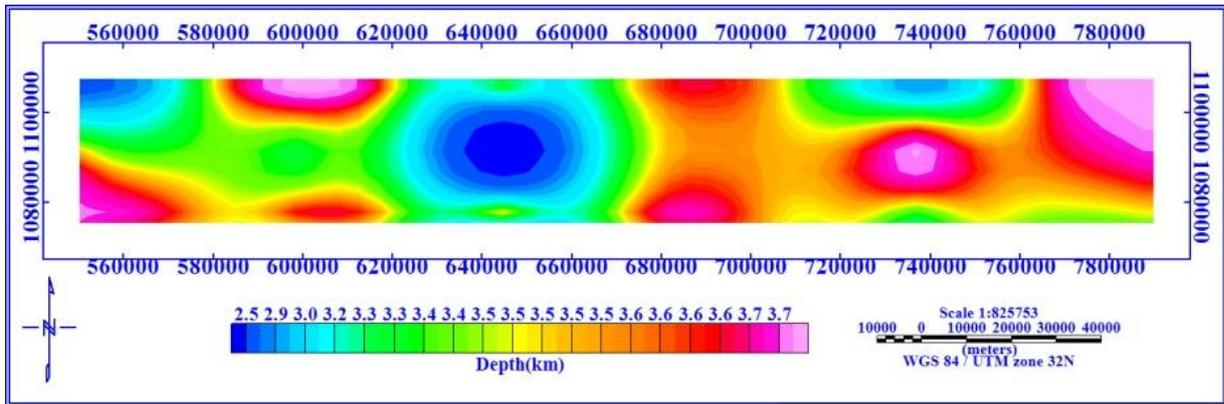
Figure 7: Aeromagnetic Depth to the bottom of magnetized body
