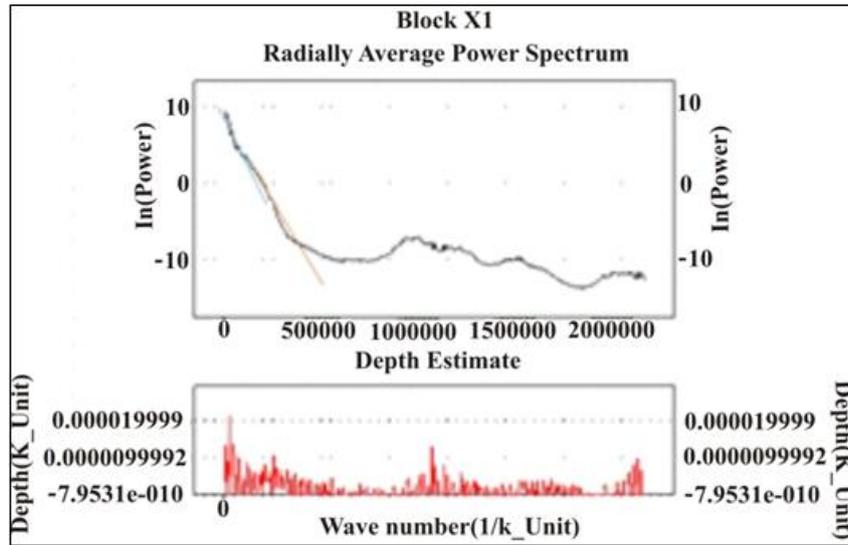
Figure 6: Radially Averaged Power for the 18 Spectral block cells (blocks 1-18) for Estimation of Depth to the bottom of magnetics source using spectral analysis.
