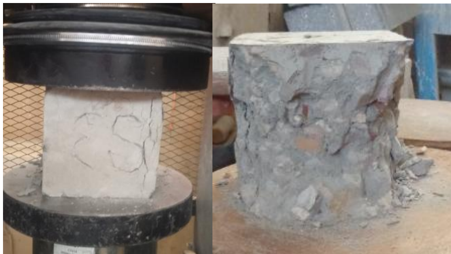
Figure 2: (a) Test cubes (b) Failure shape
