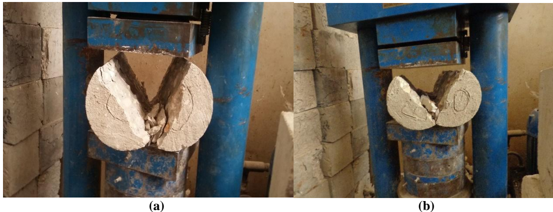
Figure 3: Failure shape of cylinder (a) 0% & (b) 50% PCCA
