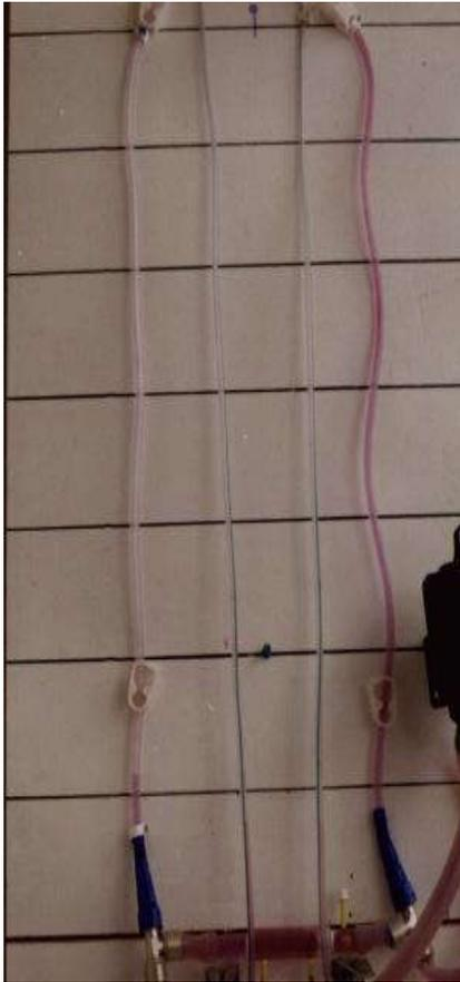
Figure 14 shows the same system of figure at (13), just by elevating the pump above the level of G tube. The DP now reads <12 cm water. PP is >70 cm water. Also, the CP in both manometers turns positive but, still lower than DP of +7 cm water near the inlet and +9 cm water near the exit. So, the flow in Chamber C is in the opposite direction to flow in the system from exit to inlet of the G tube.
