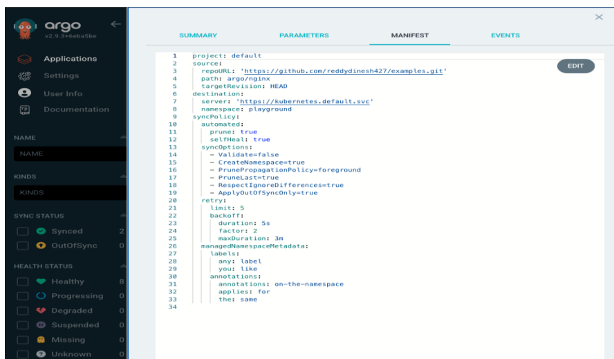
Figure 3: ArgoCD application, syncing a git repository
