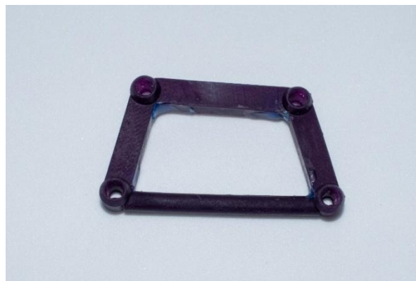
Figure 4: The bar of CastableWax ® after the supporting structure removal and obturation of the vents
