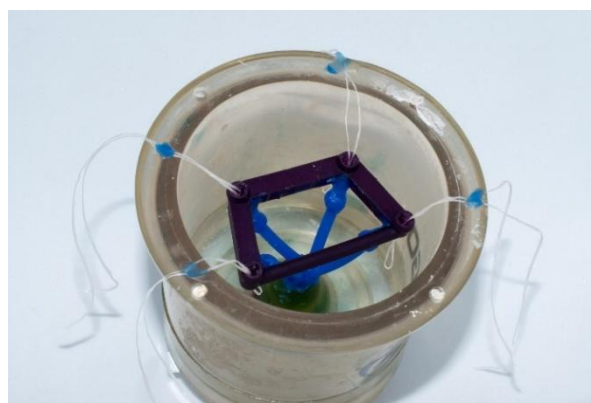
Figure 5: The bar after sprue system fabrication and fixed to the casting cone. Threads are used to remove any bubble that may appear inside the fitting surface of the bar during the investment procedure
