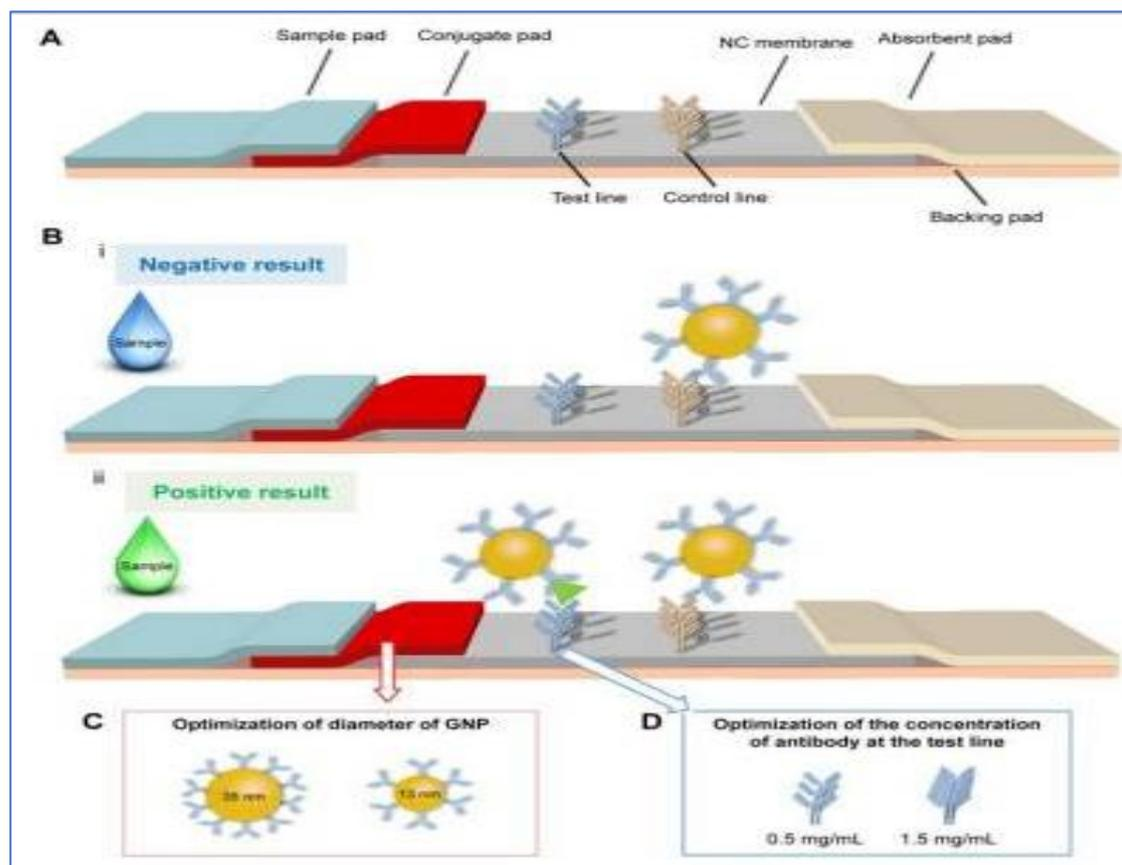
**Figure 2:** Adaption from Gong *et al* with permission.<sup>18</sup> **A**-The structure of previous LFA is adjusted by adding a conjugate pad to form a new type of LFIA. **B**-The negative result **i** – positive result **ii**-the principle of LFIA. **C**-The diameter of GNP is adjusted from 13+3 to 35+3 nm. **D**-The concentration of test line is adjusted from 0.5 to 1.5 mg/ml.
