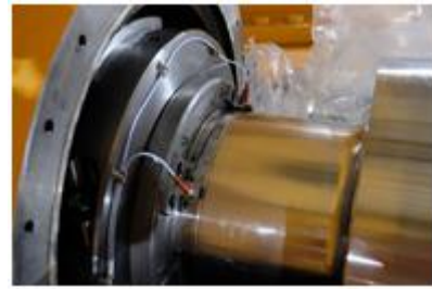
Figure 3: Sensor Installation on Turbine Bearing
