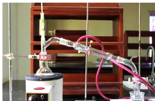
Figure 22: Extraction of the metabolite using simple distillation
