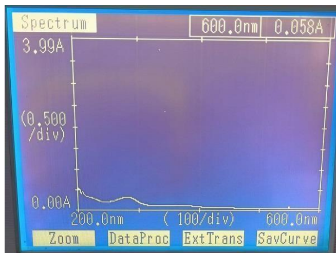
Figure 5.3: UV scan of quercetin in methanol
