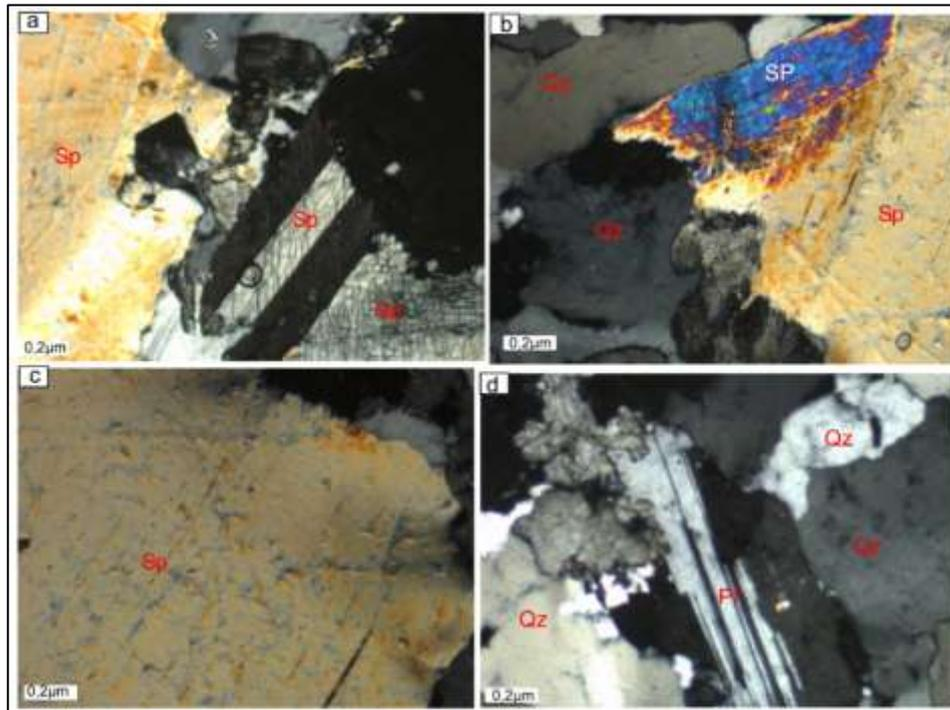
**Figure 16:** Polarized and Analyzed Light (PAL) observation of thin sections of pegmatite N° 15 (a, b, c and d). (a) Spodumene (Sp) in prismatic crystals and in patches; (b) Spodumene associated with Quartz (Qz); (c) Spodumene in patches; (d) Quartz and Plagioclase (Pl).
