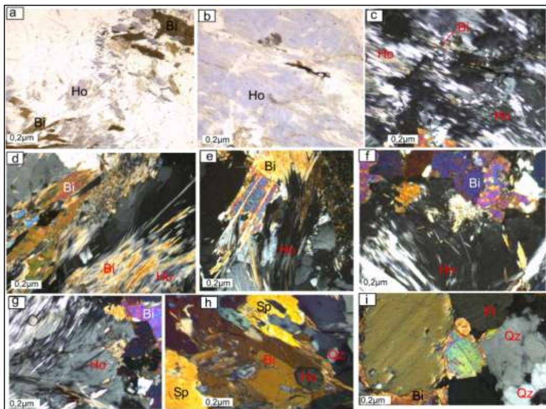
**Figure 11:** Polarized and Analyzed Light (PAL) observation of biotite - granite thin sections (c, d, e, f, g, h, and i); Polarized and Unanalyzed Light (PLN) observation (a, and b). (a, b, c, d, e, f, and g) Transformation of Biotite (Bi) into Holmquistite (Ho) by metasomatism; (h) Enrichment of the granite in spodumene and association between quartz, spodumene, and holmquistite; (i) Association between Biotite, Quartz (Qz), Plagioclase (Pl), and Holmquistite.
