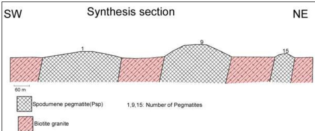
**Figure 17:** Synthesis section showing the three most mineralized pegmatites of the Dibilo field.
