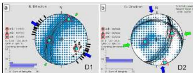
**Figure 20:** (a) Projection of the Schistosity/Foliation (S1) planes of the Dibilo area; (b) Dextral and sinistral shear corridors of the D2 phase, NNW - SSE and WSW - ENE compression, respectively.
