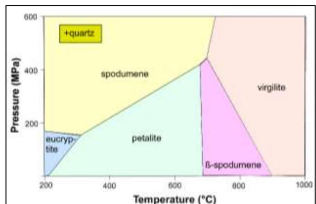
**Figure 19:** Phase diagram of lithium silicates under quartz saturation conditions [44], [45].
