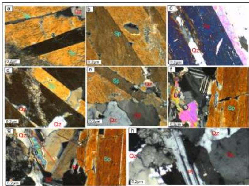
**Figure 13:** Polarized and Analyzed Light (PAL) observation of thin sections of pegmatite N<sup>o</sup>9 (a, b, c, d, e, f, g, and h). (a, b, and c) Prismatic crystals of Spodumene (Sp); (d and e) Spodumene intergrowth with Quartz (Qz); (f and g) Spodumene with Plagioclase (Pl), Quartz and Lepidolite (Lé); (h) Plagioclase - quartz.
