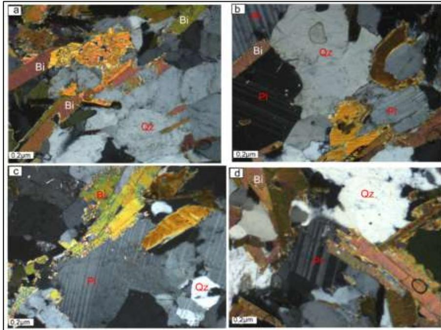
**Figure 4:** Polarized and Analyzed Light (PAL) observation of thin sections of biotite - granite (**a, b, c and d**). (**a**) beginning of foliation; (**b**) Plagioclase (Pl) and Quartz (Qz) intersect Biotite (Bi); (**c and d**) the appearance of small Quartz crystals in Plagioclase
