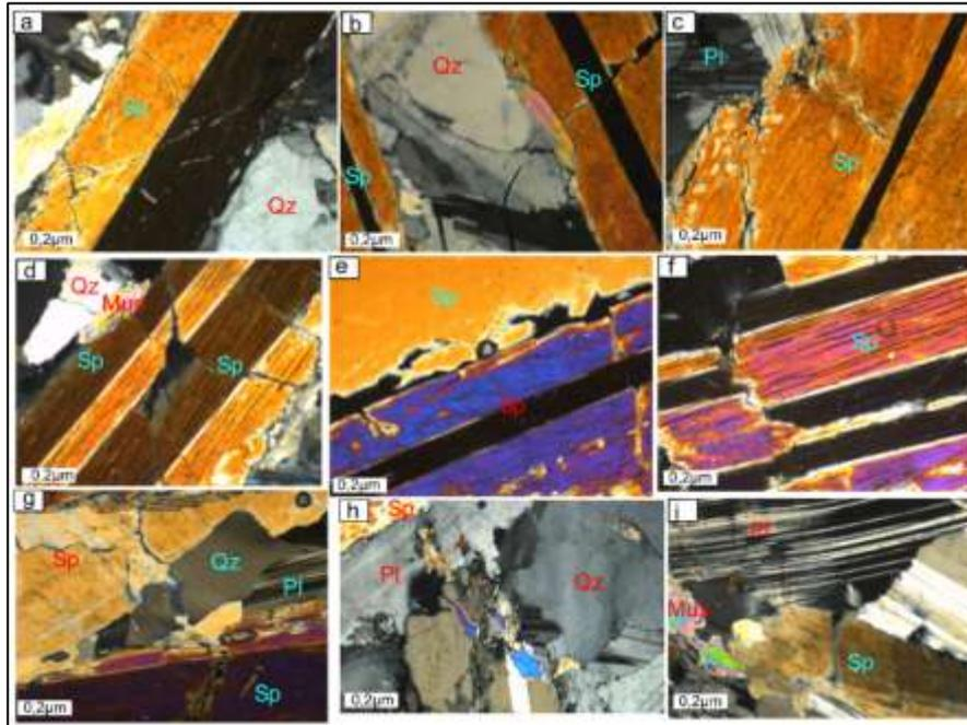
**Figure 8:** Polarized and Analyzed Light (PAL) observation of thin sections of pegmatite N°1 (a, b, c, d, e, f, g, h, and i). (a, and b) Spodumene (Sp) intergrowth with Quartz (Qz); (c) Spodumene with Plagioclase (Pl); (d) association between Spodumene, Quartz and, Muscovite (Mus); (e, and f) Spodumene; (g) Spodumene with Plagioclase and Quartz; (h, and i) Spodumene - Plagioclase - Quartz - Muscovite.
