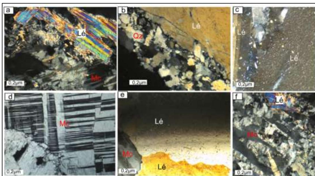
Figure 15: Polarized and Analyzed Light (PAL) observation of thin sections of pegmatite N°18 (a, b, c, d, e, and f). (a, e and f) Lepidolite (Le) and Microcline (Mc); (b and c) Lepidolite and Quartz (Qz); (d) Microcline
