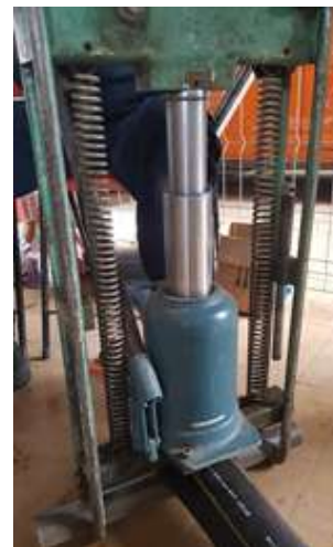
Figure 2: Squeeze-off tool used for shutting off polyethylene pipes with diameter of 63 to 160 mm
