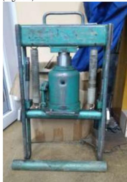
**Figure 2:** Squeeze-off tool used for shutting off polyethylene pipes with a diameter of 63 to 160 mm
