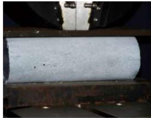
**Figure 3:** Fastening the pipe in the universal testing machine
