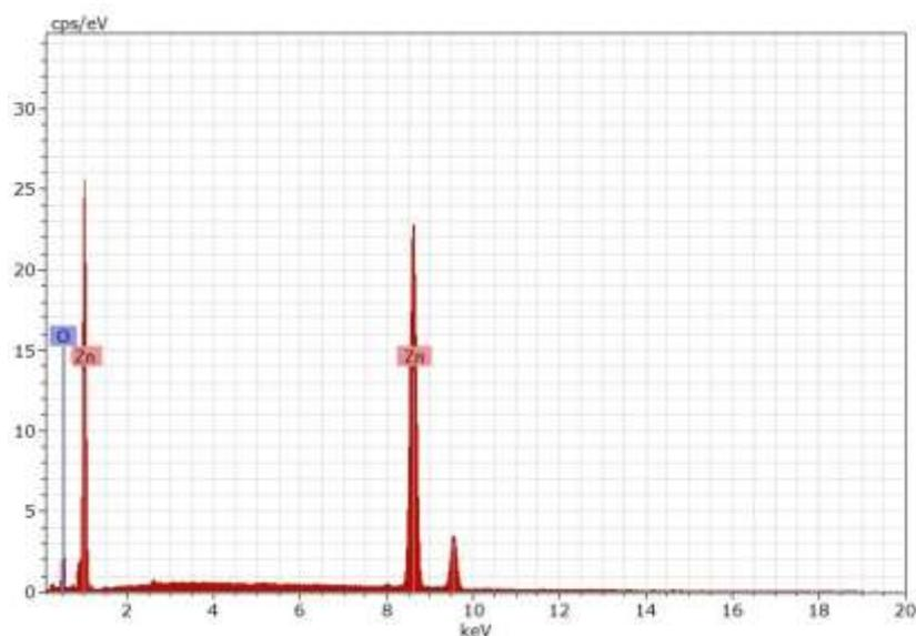
Figure 4: EDAX spectrum of ZnO thin film (600 nm)
