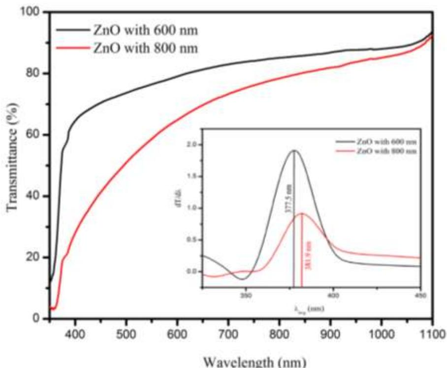
**Figure 2:** Optical transmittance spectra of ZnO thin films.
