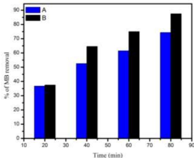
**Figure 8:** Photocatalytic degradation of MB using (A) ZnO film (600 nm) and (B) ZnO film (800 nm).
