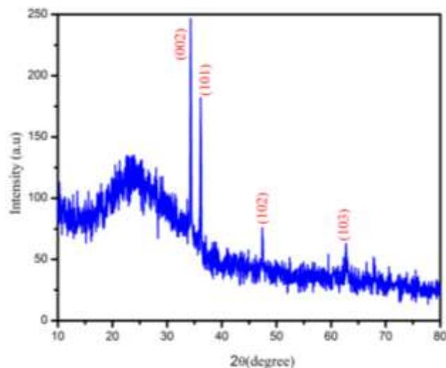
Figure 1: XRD pattern of ZnO thin film.
