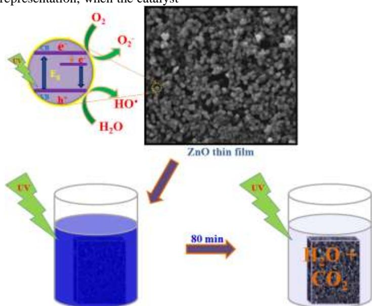
Figure 7: Schematic representation of photocatalyst mechanism of ZnO thin film
