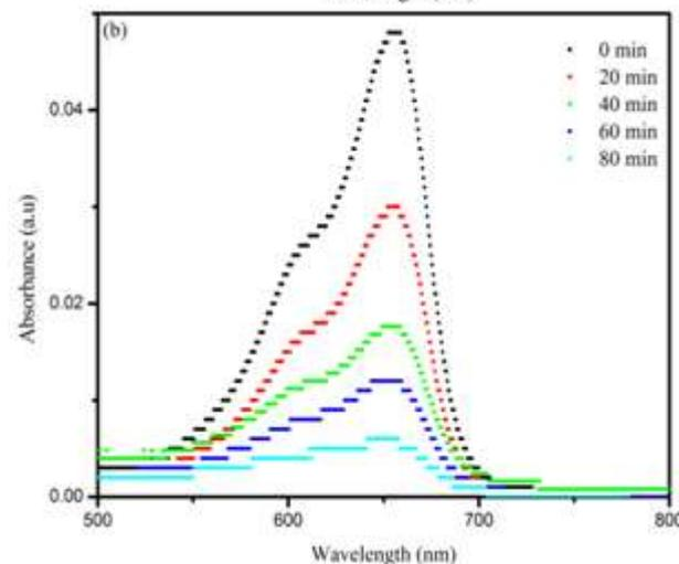
Figure 6 (a), 6 (b): Absorption spectra of MB solution in the presence of ZnO film (600 and 800 nm) at different intervals
