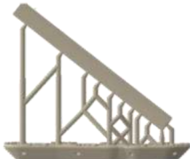
Figure 2: The diagonal oriented test samples with support structures
