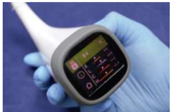
Figure 5: The measured values of a test sample - ΔE, value, chroma and hue
