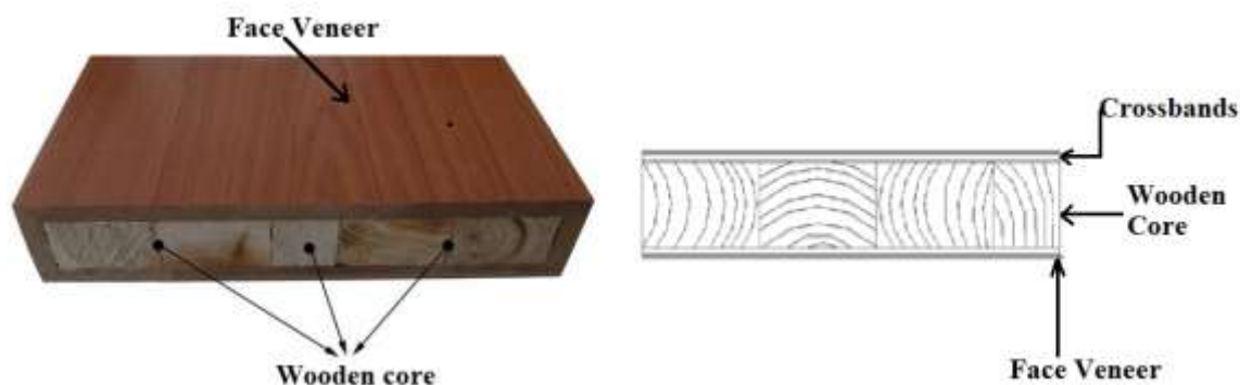
Figure 1: Cross sectional view of a Flush door
