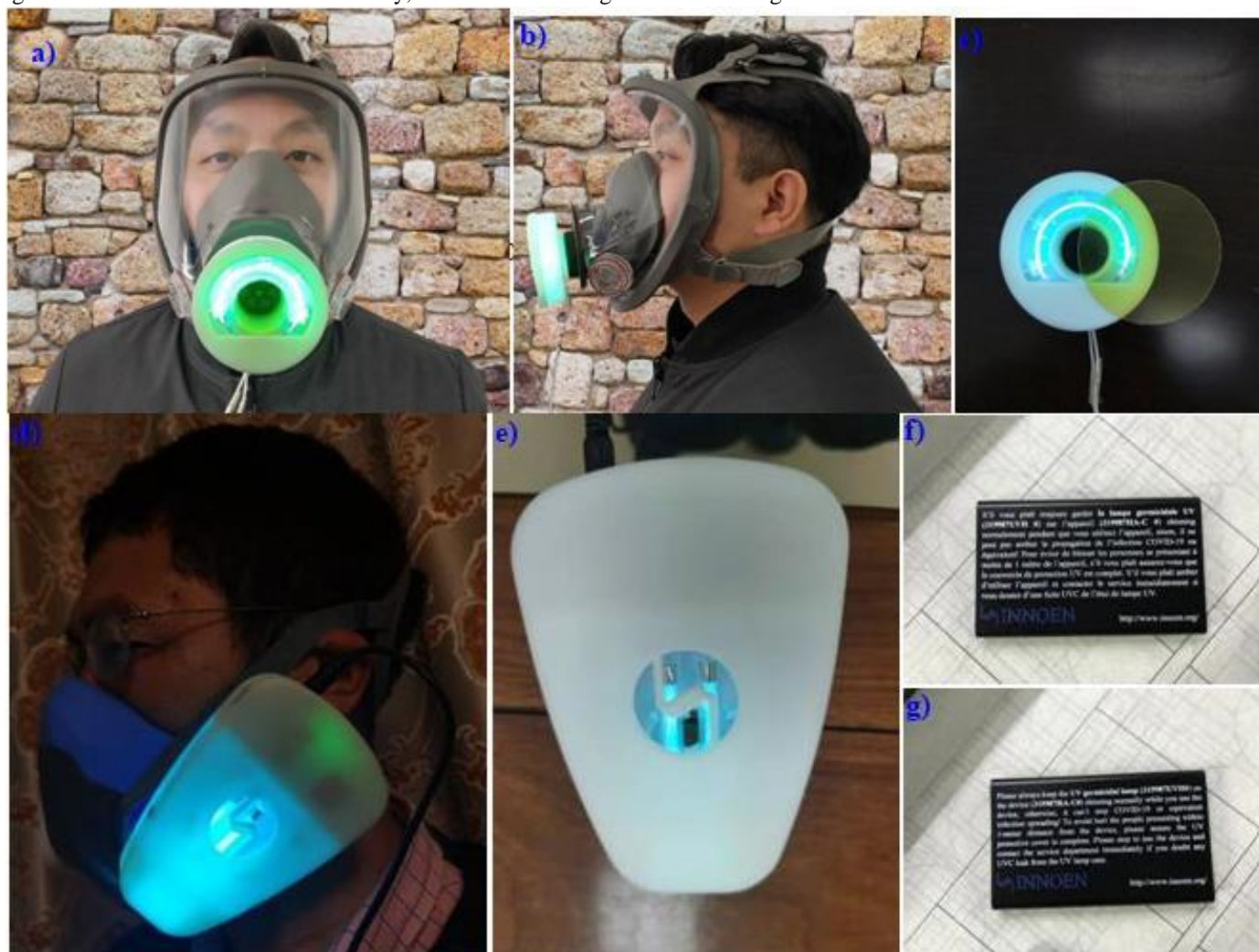
Figure 1: Innoen® COVID-19 airborne infection UV quarantine® devices (319987 HA#) and the power bank a) a 319987HA# UV quarantine® device with one set of ring-shaped UVC germicidal lamp. b) side view of it. c) a ring-shaped UV germicidal lamp housing of the device with the UVC protective cover opened. d) a 319987HA# UV quarantine® device with two sets of U-shaped UVC germicidal lamps. This type of design fits for those with glasses and also in a less infected region. However, while coronavirus concentration reaches a certain threshold, people must use devices with full eye covering like in Fig. a) & b), the latter comply with the medical device definition from regulatory affairs. We should also note while facing bio-weapons’ attack, this type of design must combine with eye goggles, human eyes are quite weak for aggressive infectious agents. e) one set of U-shaped UV germicidal lamp housing with the lamp shining inside it. f)-g) The products need a 10000mA power bank which can last for 8-12 hours. Each side of the power bank with the COVID-19 instruction on it.
