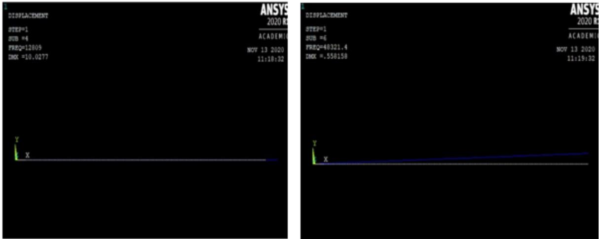
Figure 2.1.1.10: Four natural frequency mode shapes of Al-10% Fly ash composite beam
