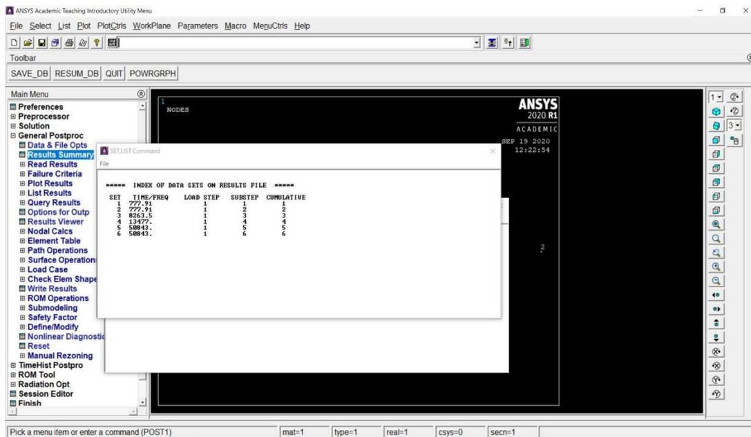
**Figure 2.1.1.5:** Modal analysis of Al-10%AV composite beam
