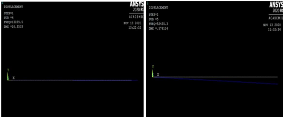
Figure 2.1.1.8: Four natural frequency mode shapes of Al-15%AV composite beam
