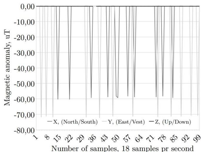
**Figure 5:** Magnetic field variation shown in the time domain. Measurements are made with a 3-axial probe and a sample frequency of 18 samples pr second. Probe frequency response is between 0 Hz and 5 Hz. Measurement resolution is 0.1  $\mu$ T.
