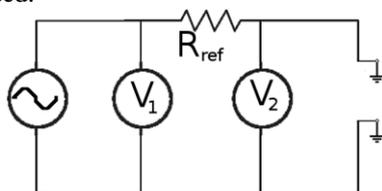
**Figure 1:** Classical I-V method diagram. Signal generator produces AC voltage, which are measured on each side of the precision resistor (500Ohm), whereby the current and impedance ( $Z$ ) between the two earthing rods can be calculated for different frequencies by measuring  $V_1$  and  $V_2$  with an oscilloscope
