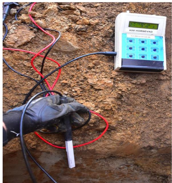
**Figure 5:** Detailed measurement of magnetic field directly on the conducting layer of ocher in an excavated magnetotelluric anomaly. In this instance a reading of 135,4  $\mu$ T (1354 mG) was recorded.
