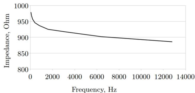
**Figure 8:** Impedance, measured in Ohm, for the frequency range between 40 Hz and 13000 Hz.
