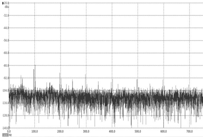
**Figure 7:** 0 Hz to 750 Hz spectrum analysis from magnetotelluric anomaly. Note the peak around 1Hz which possibly is related to the peaks with a quasi-frequency around 1Hz shown in figure 5. Note the double-peaks around the mains frequency (50Hz). Note the broad peak around 180Hz.
