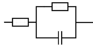
**Figure 10:** Equivalent circuit for the impedance observed at the magnetotelluric anomaly.
