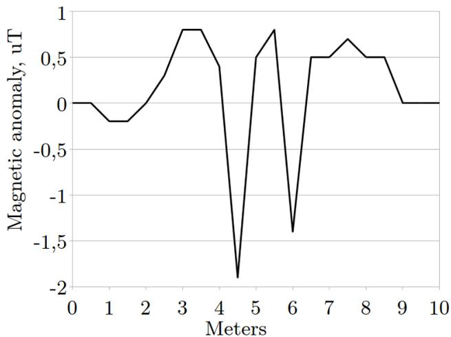
**Figure 3:** Cross-sectional magnetic field survey “1” Measurements are taken with an axial probe, whereby only the “Z”-component (perpendicular to the surface) is registered. Frequency response of the used probe is 0 Hz to 5 Hz. Measurements were taken for each 0,5 meters. 10 seconds of measurements were taken at each station and the average recorded.
