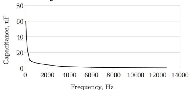
**Figure 9:** Capacitance, measured in uF, for the frequency range between 40 Hz and 13000 Hz.
