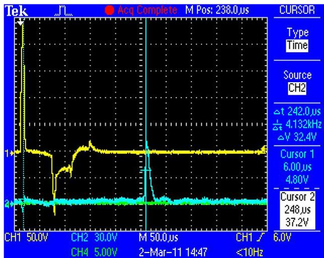
**Figure 1:** CRO Signal of velocity probe system (Ch-1 and Ch- 2 shows signals received by probe-1 and 2 respectively)
