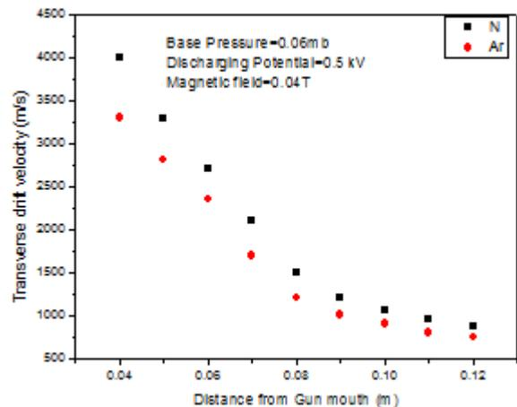
**Figure 3:** Spatial drift velocity of argon plasma in a curved magnetic field (~0.04T) at discharging potential 0.5 kV and base pressure 0.06 mb.
